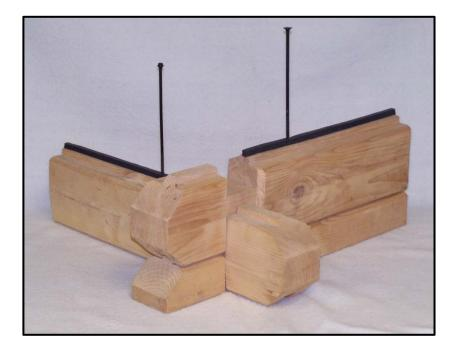
Our interlocking design increases the overall strength and durability of our log cabins. It also provides a weather tight seal. No leakage! Every log is kiln-dried and treated with stain on the outside and polyurethane on the inside. We also put insulation strips on every course to provide a weather tight seal.
